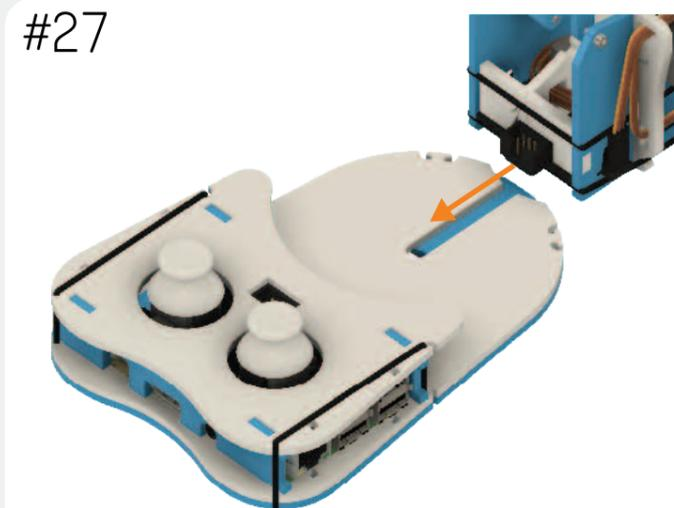
Gently prise the two base plates apart and slide the servo arm in between them and slide it down the central slot until it clips into place in the hole in the bottom
