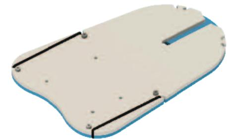
**#26b** Stretch the elastic bands over the sides of the base to use as feet
