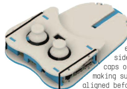
**#26c** Fit the cover over the tabs on the sides and stretch an elastic band over each side. Push the joystick caps on to the joysticks, making sure they are properly aligned before pushing
