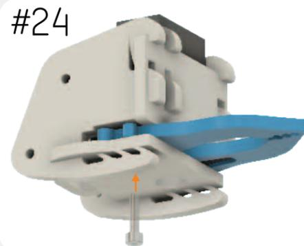
**#24** Slide the grip base (part #22) on so that the large hole aligns with the servo arm side and screw it into place through the right grip with a 10mm screw
